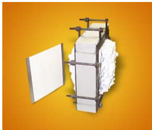
Figure 1. Commercial intumescent coating specimen prior to (left) and after testing in the slug calorimeter high-temperature experimental setup at NIST.
