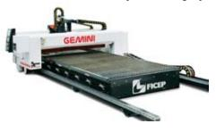
spindle (8,000 rpm) with an automatic tool changer and ball screw feed. To increase productivity, the system includes a secondary "X" axis so the spindle can position
