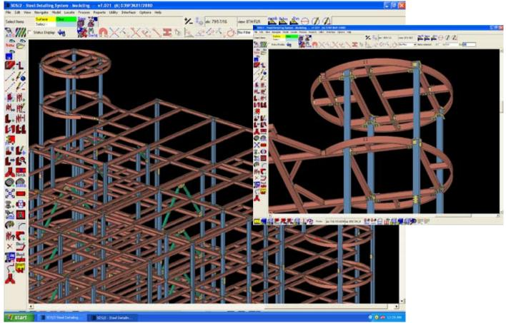
The amount of detail included in the 3D model—including much data that is not visible here—meant that the PowerHouse BIM could be consulted for many of the questions that otherwise would have become RFIs.
