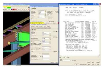
Figure 3: Properties and load calculations for a selected member are available at the reviewer's fingertips as a part of the 3D model.
