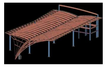
Figure 2: Individual elements of this information-rich 3D model of curved framing are shown as they relate to the rest of the structure, rather than as individual, isolated 2D drawings.
