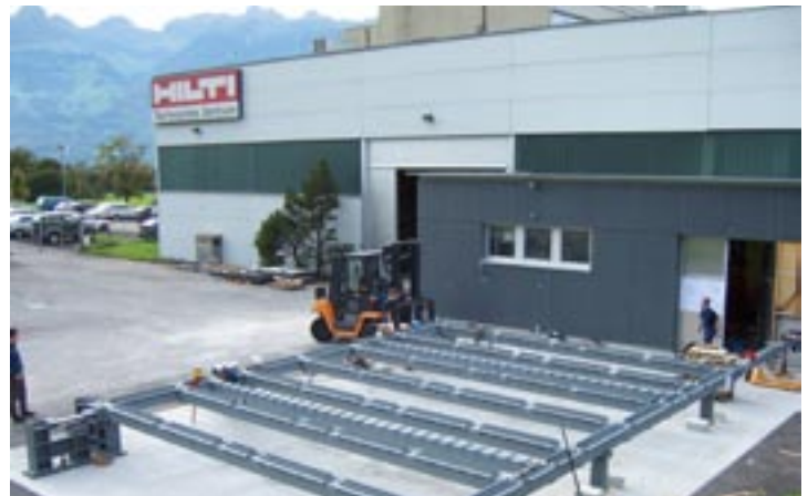
The test frame at the Fastening Systems Research Center in Schaan, Lichtenstein, simulates cyclic and seismic loading on an installed steel deck diaphragm.
