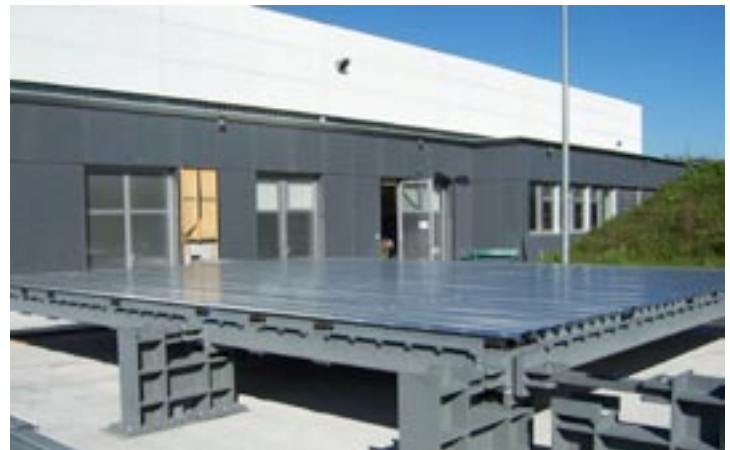
The test frame at the Fastening Systems Research Center in Schaan, Lichtenstein, simulates cyclic and seismic loading on an installed steel deck diaphragm.
