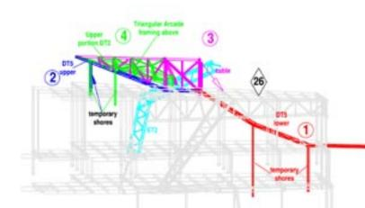
Erection plan drawings were generated by working with individual pieces and assemblies from the 3D model. Note the inclusion of temporary shores and cable attachment requirements.
