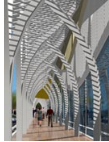
Above and below: The curved, columns are set orthogonal to the front of the building, giving the appearance of palm-like arches as one looks down the liwan (colonnade).
