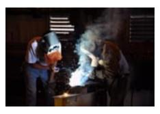
▲ Learn. An inspector uses a stopwatch to measure the welding speed per single pass of a new weld procedure. The photo was taken in Herrick Corporation's Stockton, Calif., shop.
