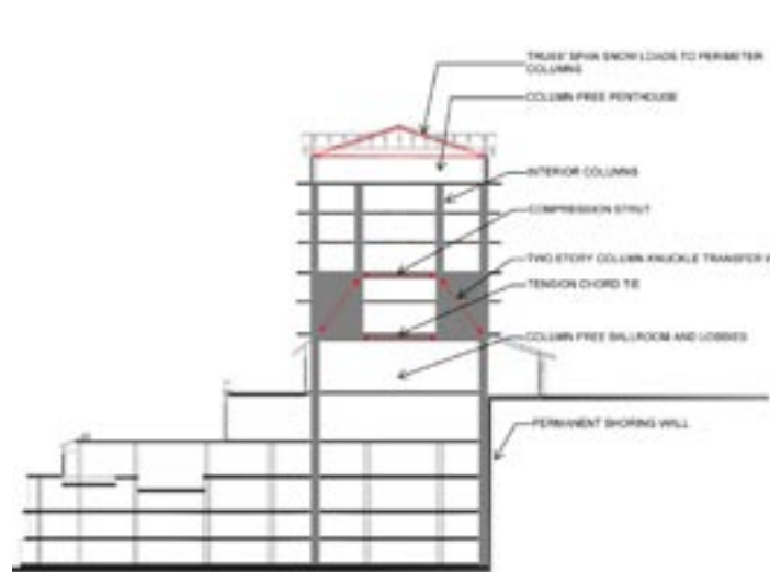
▲ Building cross section of column transfer.
