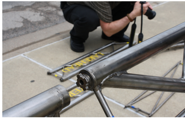
▲ The “camera connection” developed by the Lakehead University steel bridge team was both very efficient in transferring loads and quick to assemble.
