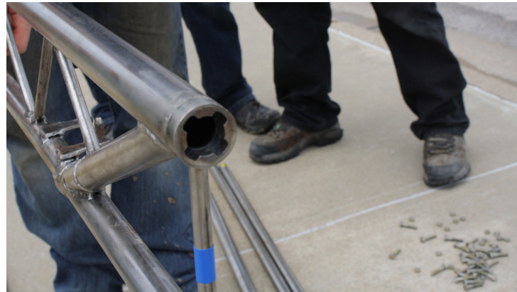
▲ The “camera connection” developed by the Lakehead University steel bridge team was both very efficient in transferring loads and quick to assemble.
