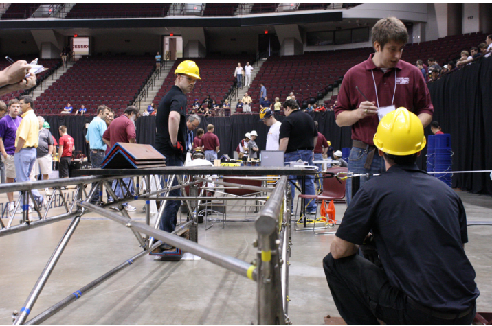
▲ Measuring the Lakehead University bridge's horizontal deflection.
