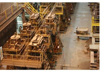
A Continuous caster molds for wide-flange shapes at the SDI mill.
