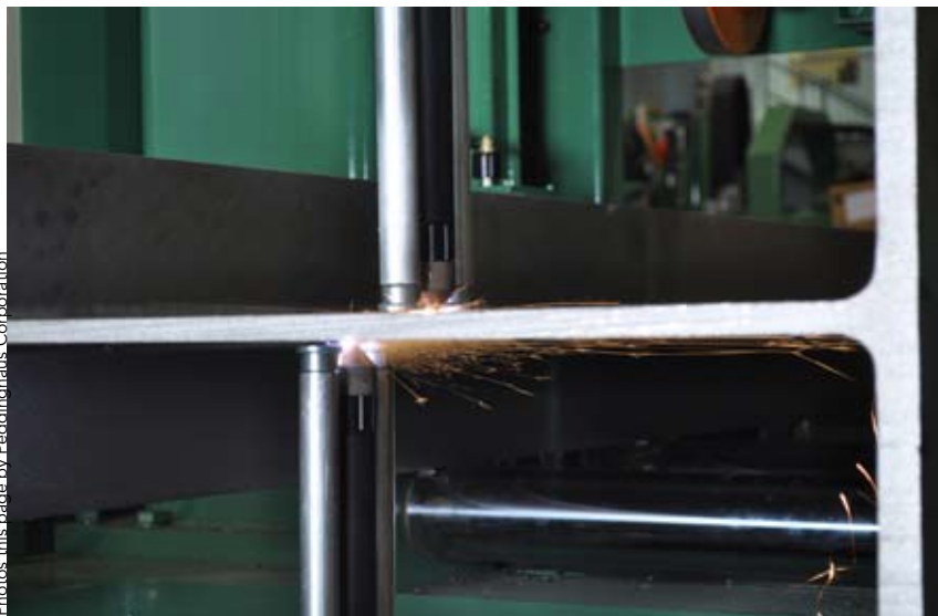
▲ Above, center and below: The PeddiWriter uses a plasma torch to mark the surface of the steel.
