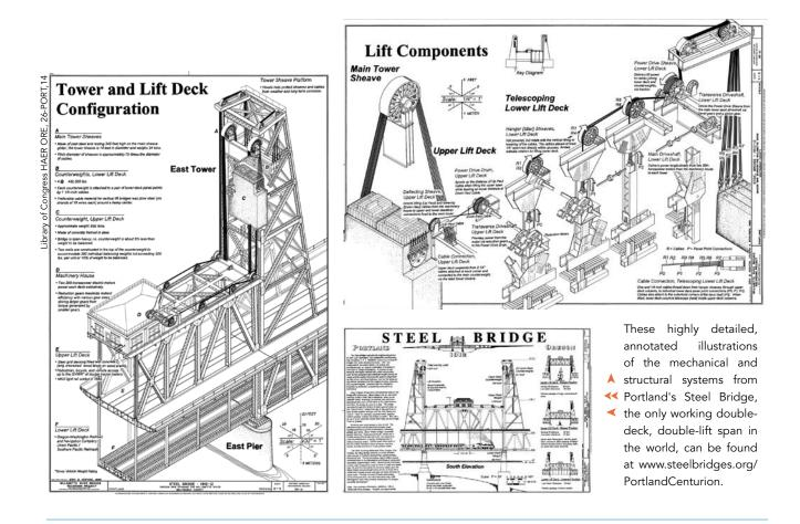
290 and 300-ft long, complete the river crossing. The typical top deck width runs to 74.5-ft (62.5 ft for the roadway plus two 6-ft sidewalks). The sidewalks flare out at the towers, taking the maximum width to 77 ft.
