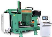
tions for plate/angle connections, welding, part identification, crane lifting points and more can be processed in a fully CNC method. In addition, by marking on all four sides at once, it eliminates expensive crane lifts.
