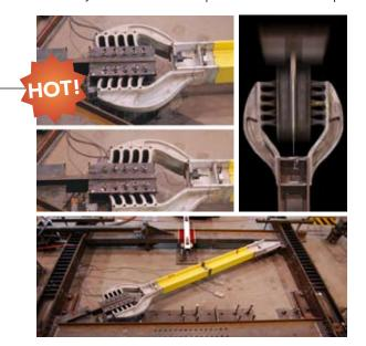
vertical truss system that resists lateral forces. YBS have more ductility and energy absorption than SCBF/Type-MD CBF because overall brace buckling and its associated strength degradation are eliminated.
