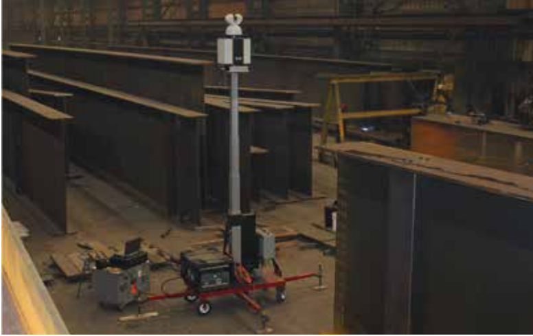
◀ VAS measuring a girder in a fabrication shop.
