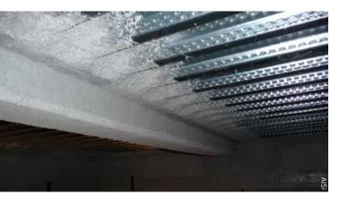
An unrestrained steel-framed floor specimen, before and after the fire test.
