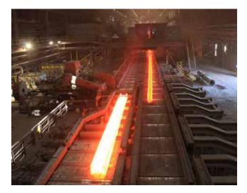
Steel exiting the breakdown mill (left) and being rolled in the universal rougher/edger mill (right).
