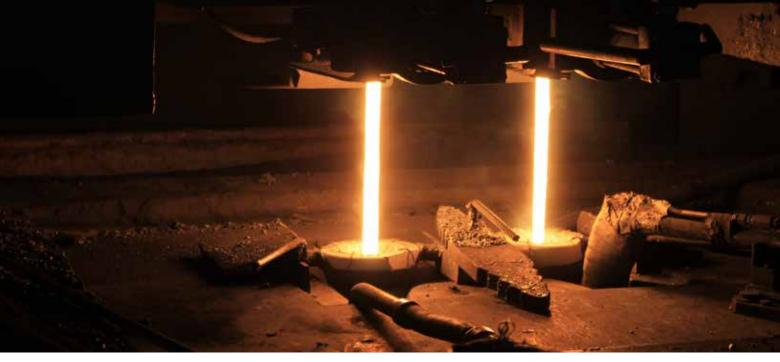
Casting the steel. Two molten steel streams are fed into molds. Granulated powder is also continuously fed into the molds so that the steel doesn't stick—much like greasing a pan.
