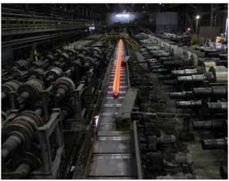
After going through all three sets of rollers, each one further forming the shape, steel is ready for final cutting.
