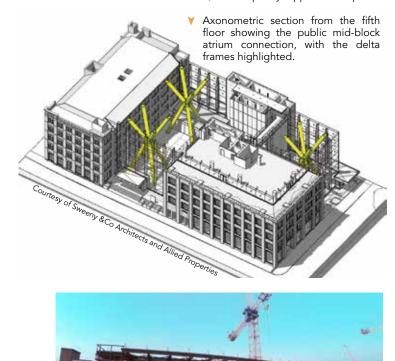
developed collaboratively with Sweeny to deliver the delta frame's resulting aesthetic, one where each of the legs appears to effortlessly curve while subtly merging with each of the neighboring legs.
