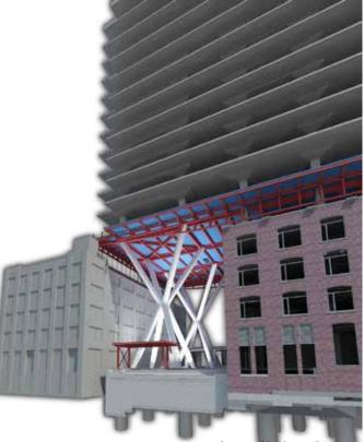
constructing the tabletop and its support from structural steel eliminated the need to shore the tabletop 70-ft above street level during construction.
