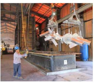
Smaller elements, such as bolts, go through the galvanizing process in special spinner baskets in the 23-ft tank. After the zinc dip, the baskets are spun in a special machine to remove the excess zinc.
