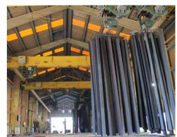
The smaller building employs 7.5-ton cranes while the larger building uses 10-ton cranes to move steel batches down the line. Each batch is tagged for tracking purposes, but the tag is attached high enough so that it is not submerged in any of the tanks or kettles.
