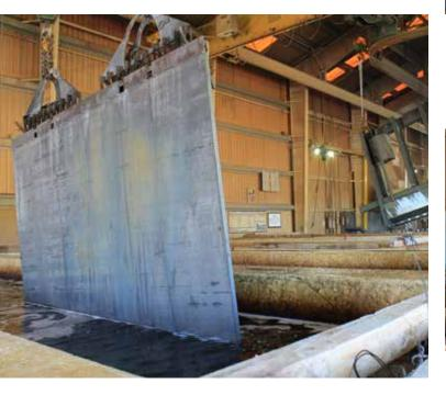
Zinc arrives at the facility in approximately 2,400-lb pieces and is added to the kettles regularly as the levels get low; the operators keep the level 2 in. to 3 in. below the lip of the kettle to prevent spillage when elements are dipped. This facility has three kettles in two different buildings, as well as a decommissioned kettle. The two longest kettles—43.5 ft long and 36 ft long—are both 6 ft wide and 9 ft deep, while the third kettle is 23 ft long, 3 ft wide and 6.5 ft deep.
