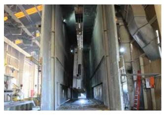
A The galvanizing process was discovered in the 1700s and the basics haven't changed much since. The mixture that the steel is dipped in is 99% pure zinc, along with a small amount of aluminum (which gives it a shine) and other proprietary chemicals.
