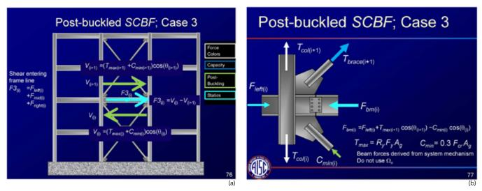
🗼 Figure 2 (a and b). Determination of post-buckled SCBF connection forces from the "Where Did that Force Come From?" webinar.
