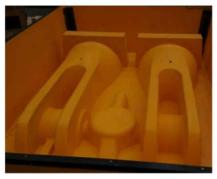
Tooling for a universal pin connector casting.
