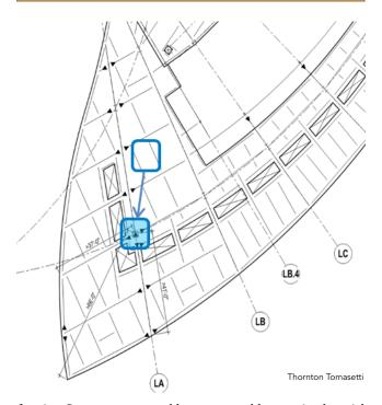
framing. In most cases, steel beams were able to resist the axial diaphragm forces without upsizing and with fairly modest impact to their extended shear plate connections.
