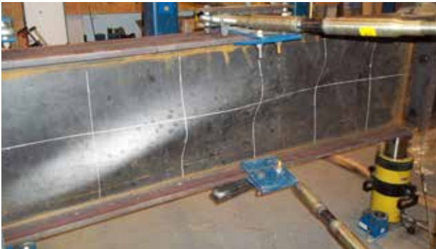
▲ Web shear buckling.
