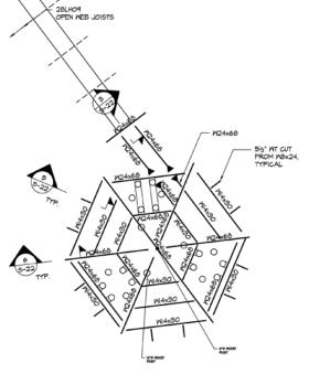
between the bridges and main structure, and specially designed connections of wood to steel posts and beams were developed to meet the connection challenge.
