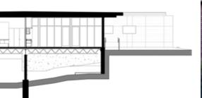
The floor framing consists of openweb steel joists and steel beams supporting concrete-over-steel deck at the interior spaces and wood deck framing at the exterior spaces. Perimeter infill walls are a combination of rammed earth, glass and clad stud walls. The lateral force resisting system for the building relies on a combination of steel moment frames, rammed earth walls and diagonally braced steel stud walls. AISC member SNC Engineering, Inc., performed the steel detailing.
