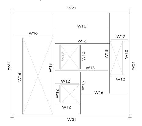
This framing plan will be difficult to erect. Looking at the sequence of erection, the W18 and two W16 beams can easily be lifted into place. However, it would not be possible to erect the remaining beams in this bay without some additional temporary support provided by the erector.
