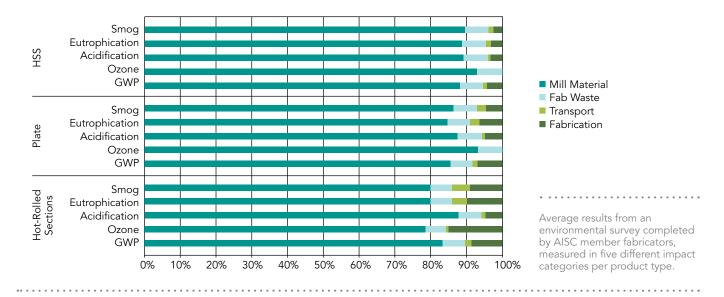
model of the steel production process, with all inputs related to materials, water, consumables and energy included for each type of steel product (hot-rolled sections, plate and HSS).
