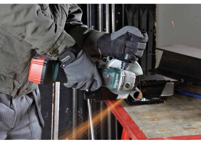
figure 3. When working with angle grinders, always secure your work with the proper vise or clamp, and don't overreach.
