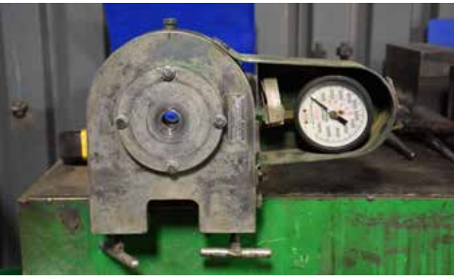
Demonstrating the Skidmore test at GDI.
