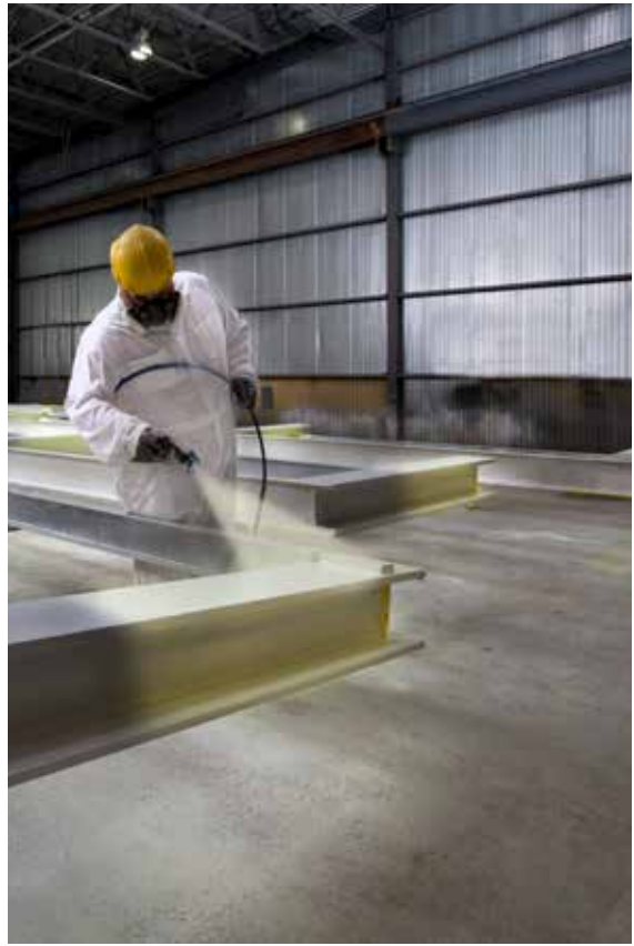
Tnemecc offers a non-structural thermal break product that can be sprayed directly onto steel in a shop environment.
