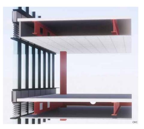
above: The office tower design allows for 9-ft, 6-in. office ceilings within a floor-to-floor height of 12 ft, 9 in.
