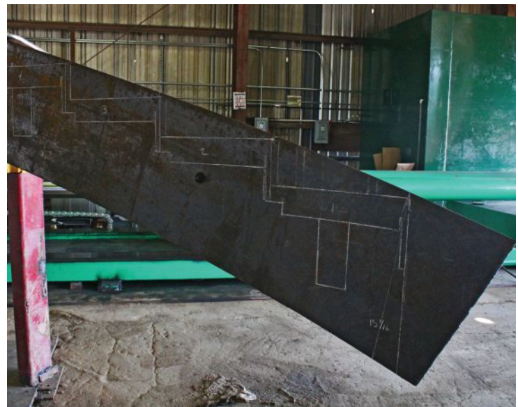
A curved stair stringer with markings for the treads and risers.
