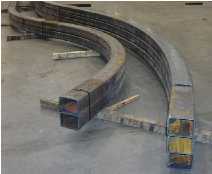
Rectangular HSS displaying reverse-compound bends.
