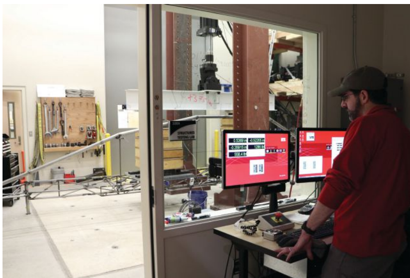
above: Observing the buckling testing operation.
