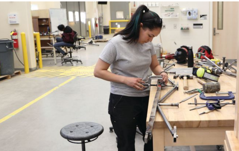
above: Assembling a truss during the fabrication stage.
