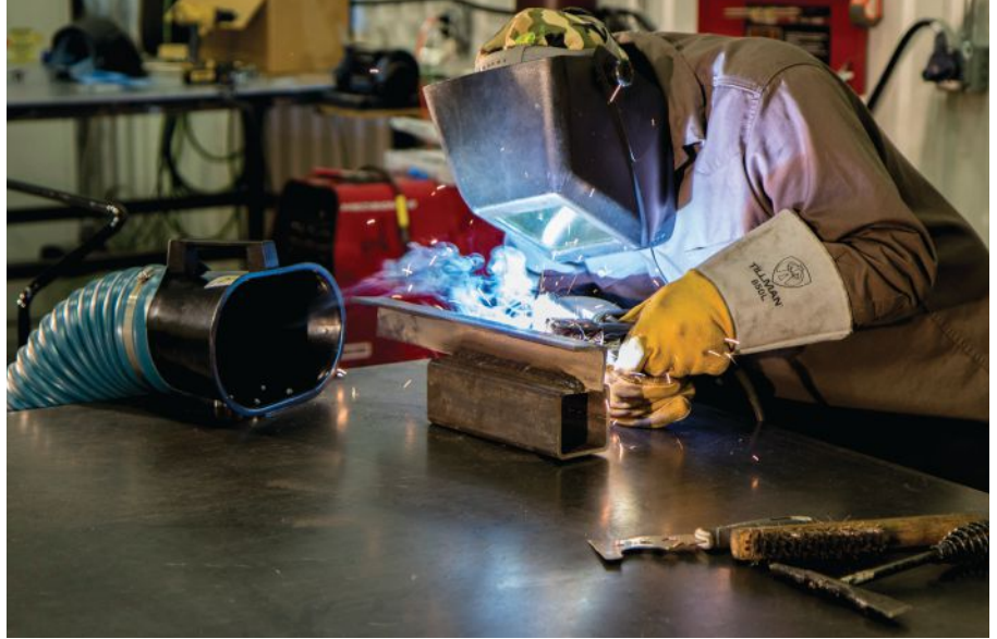
above: A portable fume extractor with an extra flexible capture hose to enable placement in hard-to-reach areas, being used beside a welder.
