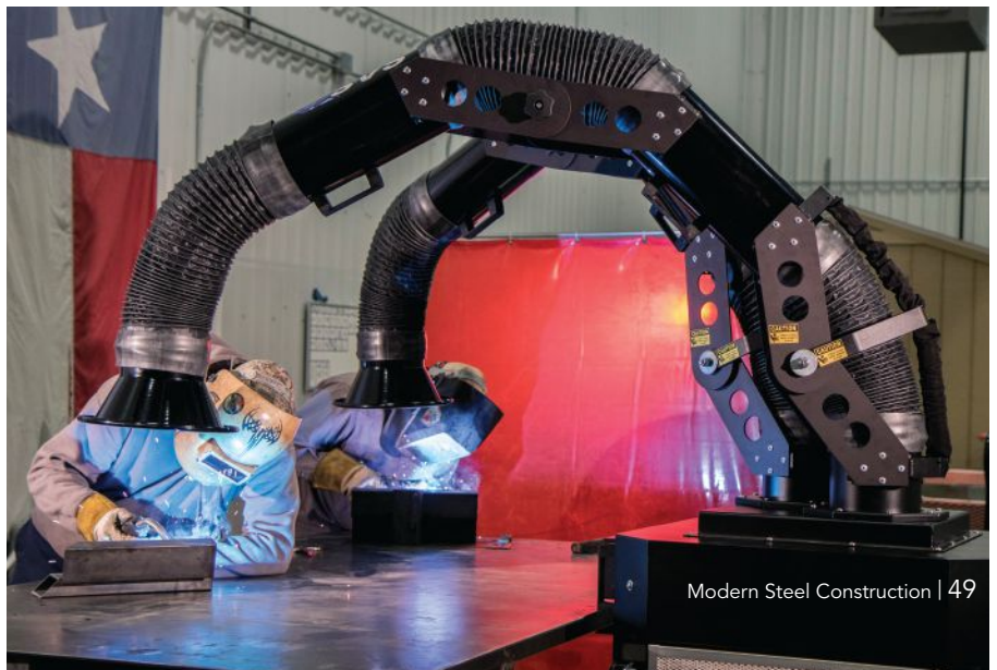
below: Two welders benefit from using a dual-arm portable fume extractor with a cleanable filter.
