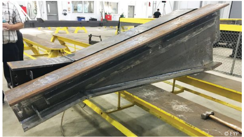
above: A tapered beam used to create the “academic main street” joining the existing building to the new atrium space. These beams are welded to and cantilever from existing columns. The existing beams are W33s, so W33s were also used for the academic main street to simplify moment connections at the cantilever. The beams are tapered from 33 in. to 6 in. so that the end of the cantilever looks thin when viewed from the atrium space.
