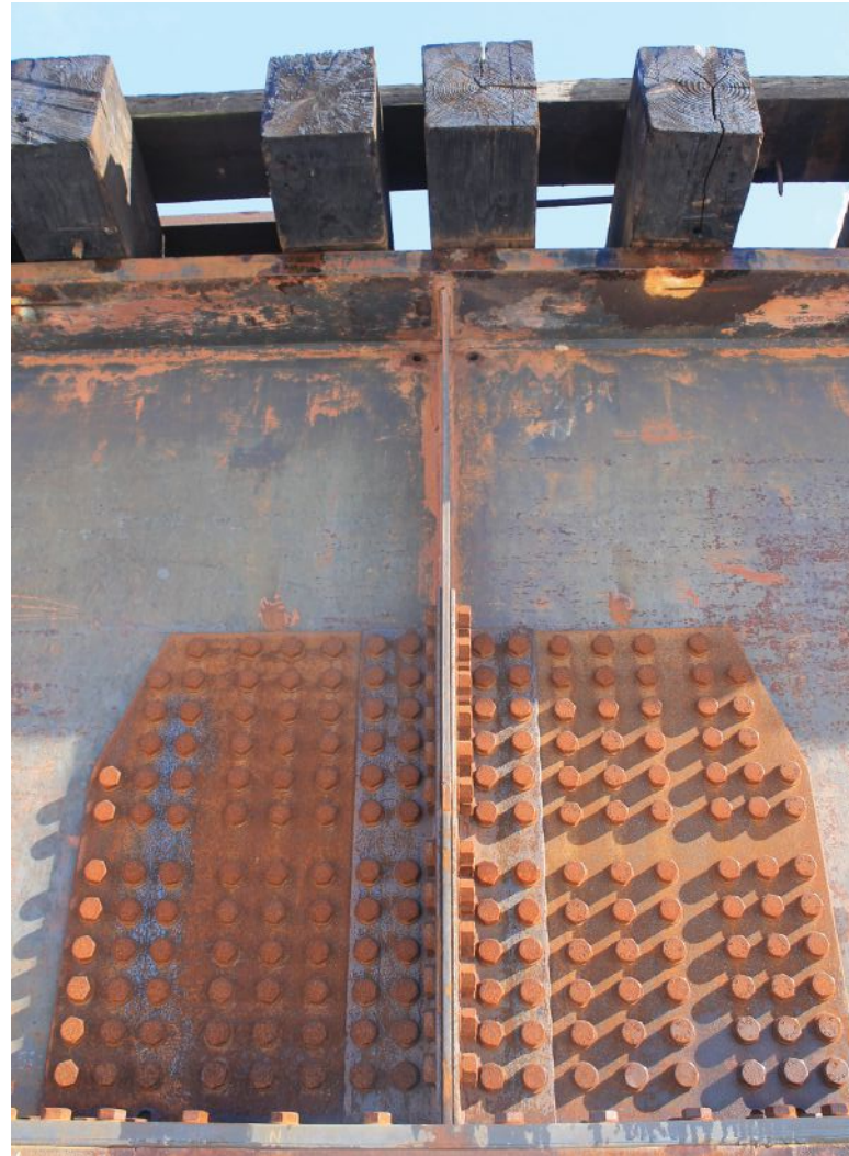
above: The first statistically significant probability of detection (POD) study for visual inspection of fatigue cracks was conducted at S-BRITE. Weathered painted specimens are shown on the left, and uncoated weathered specimens are on the right.
