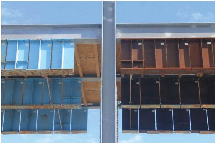
above: The first statistically significant probability of detection (POD) study for visual inspection of fatigue cracks was conducted at S-BRITE. Weathered painted specimens are shown on the left, and uncoated weathered specimens are on the right.
