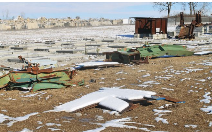
above: S-BRITE also contains many miscellaneous bridge components, such as these from the I-35W collapse.
