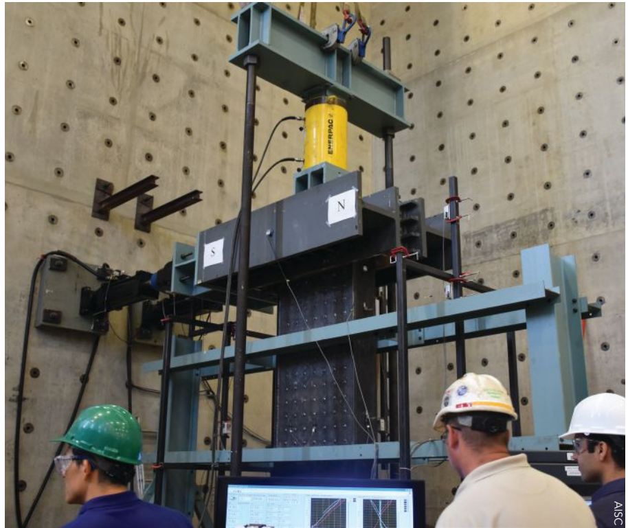
A SpeedCore prototype specimen being tested for behavior under axial and wind loading at Purdue University.
