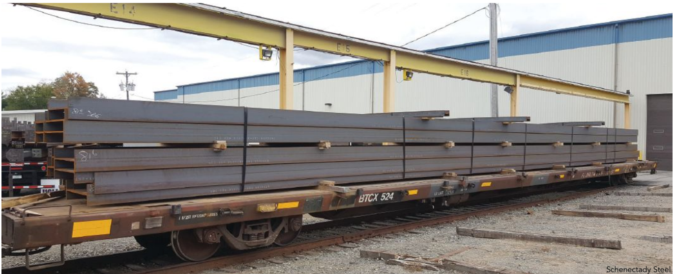
Beams were shipped from the fabrication shop to the site via rail in lengths up to around 80 ft long.
