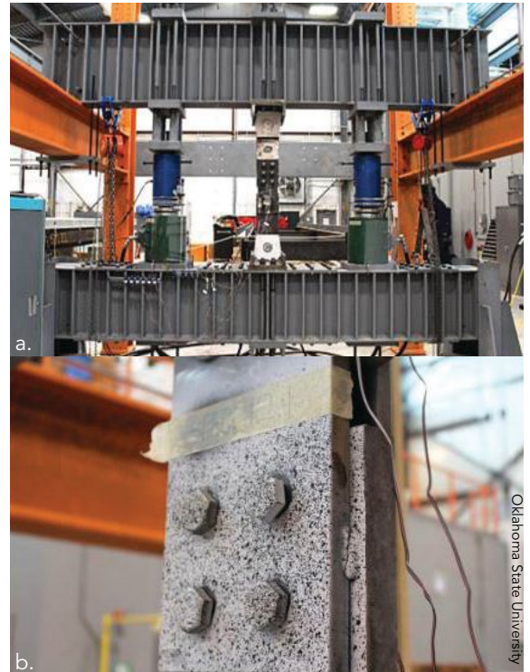
The overall setup for testing combined bolt and weld specimens (a) and a close-up of the tested specimen (b) at Oklahoma State University.
