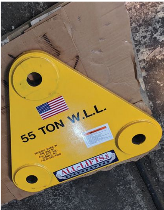
below: A below-the-hook lifting device with identifying information per ASME B30.20 section 20-1.2.1
