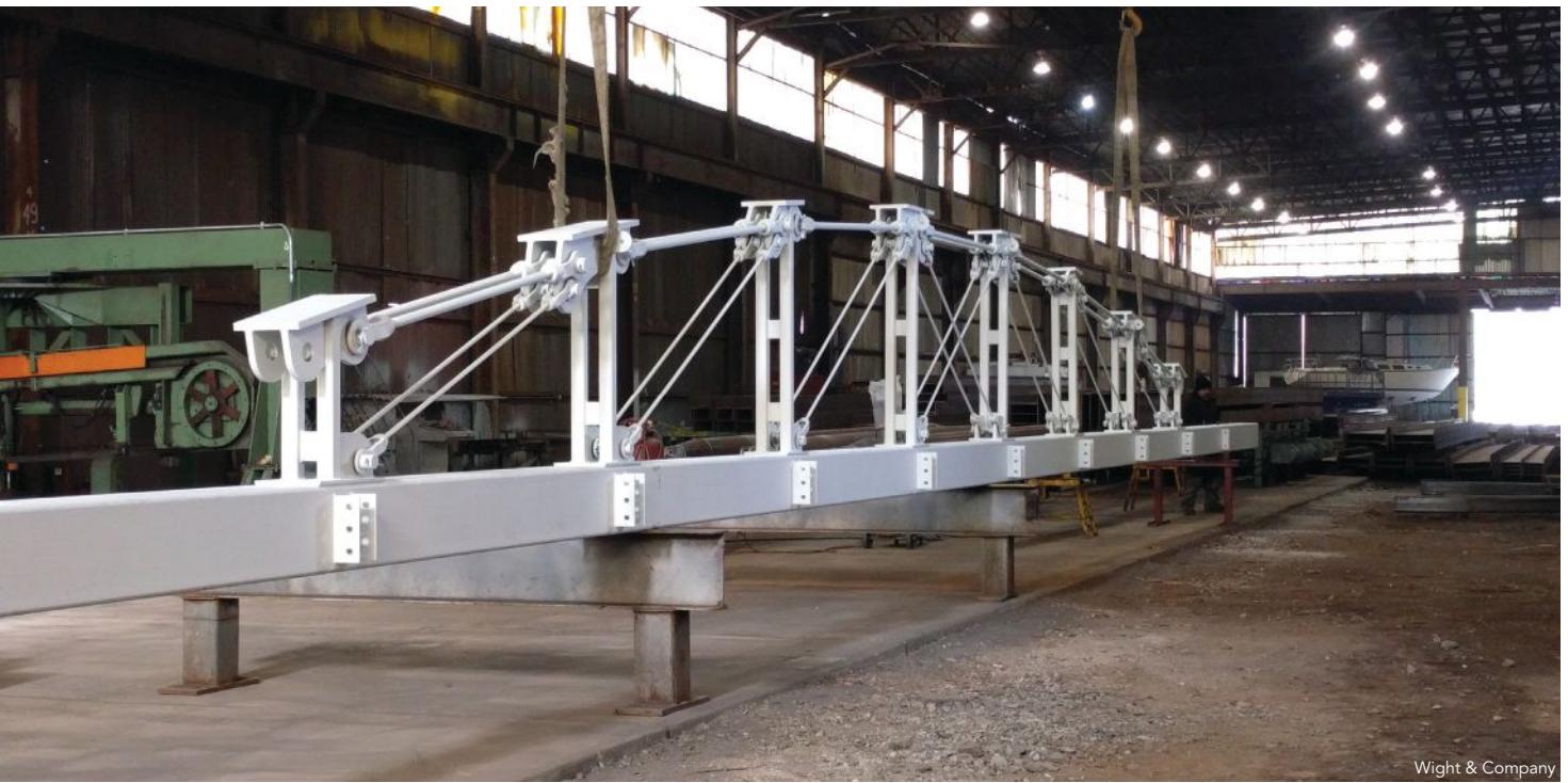
above, left, and below: Roof framing trusses—shown in the shop, in a 3D model, and installed—were designed to invoke the cable-and-strut construction of vintage airplanes.
