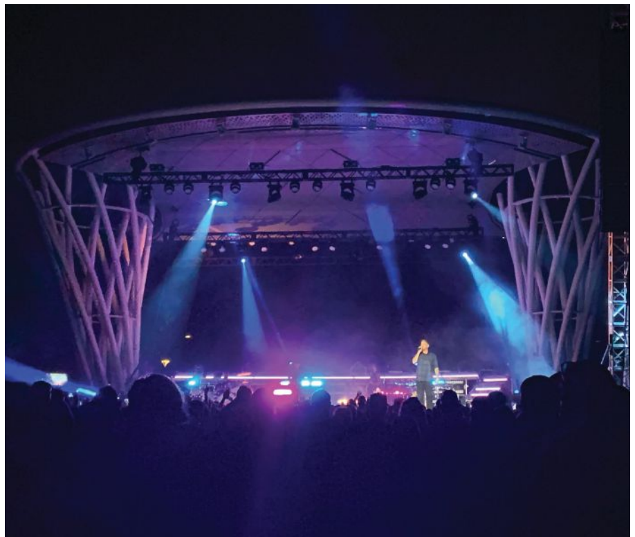
above and right: The complex, curved steel column assemblies are a natural response to the local environment, inspired by the form of an oak tree. Each weighs 13.5 tons.
