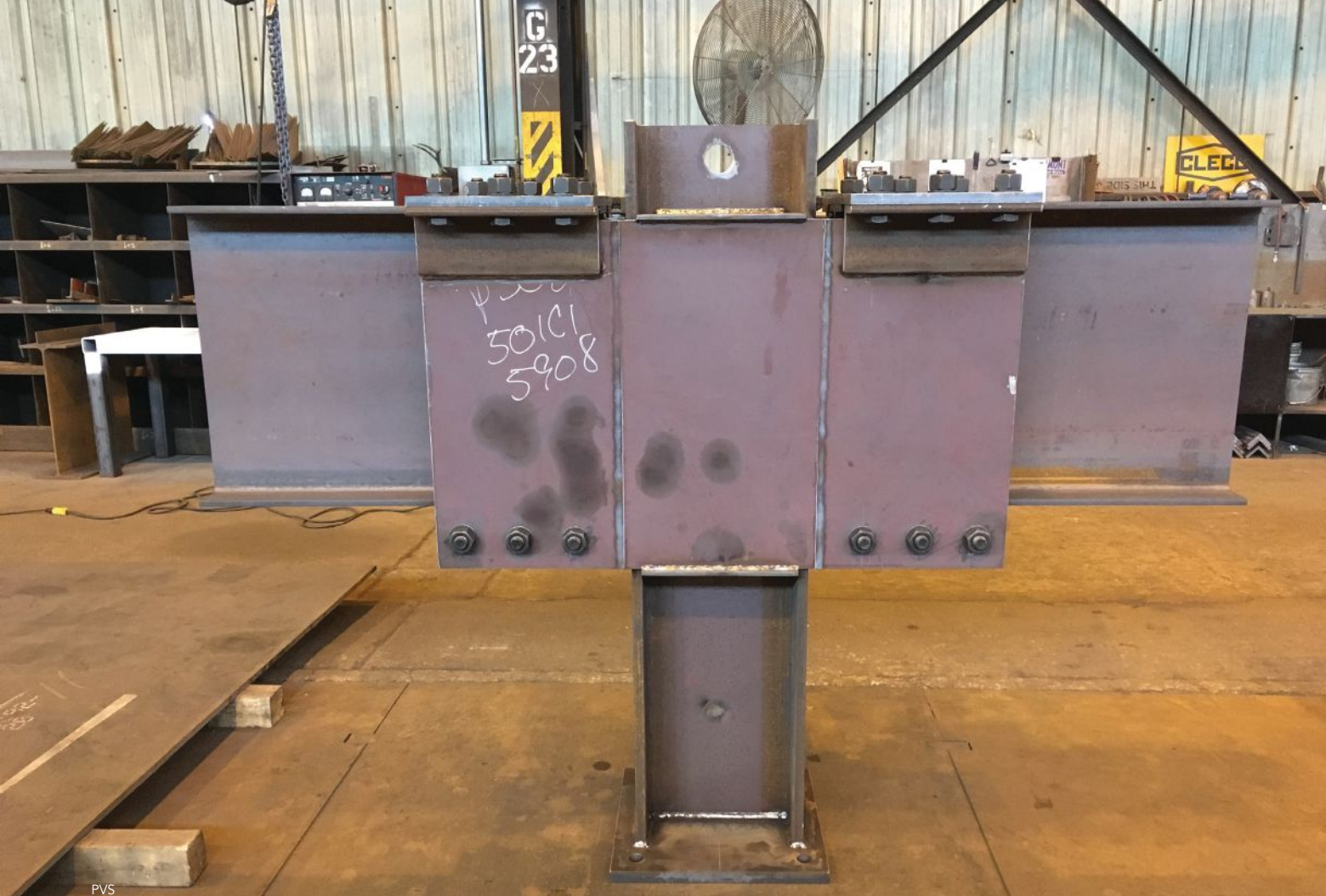
above: As this was Nebraska's first SidePlate system, steel fabricator Paxton and Vierling Steel (PVS) built a mock-up of a SidePlate connection in its shop to review constructability issues.
