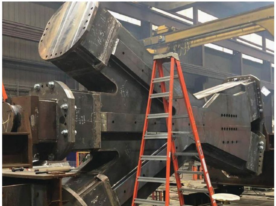
Fig. 2c. The as-fabricated weldment.
