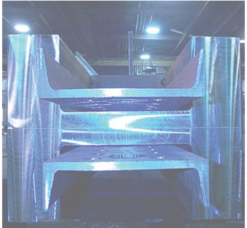
Heavily loaded compression joints for columns and trusses can often be spliced most easily using a "finish to bear" joint.
