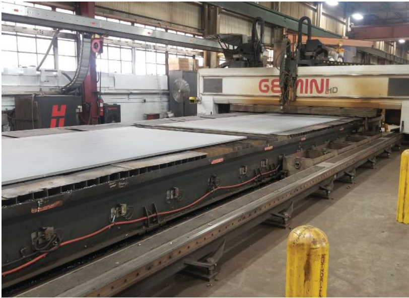
Fig. 8. A CNC plate processor (left) was used to make the three-girder cap plate diaphragms and connection plates (right).
