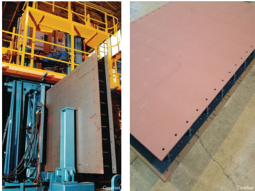
Fig. 5. A Friction-stir welding tool (left) to fabricate a bi-steel panel and a completed fabricated panel (right).
