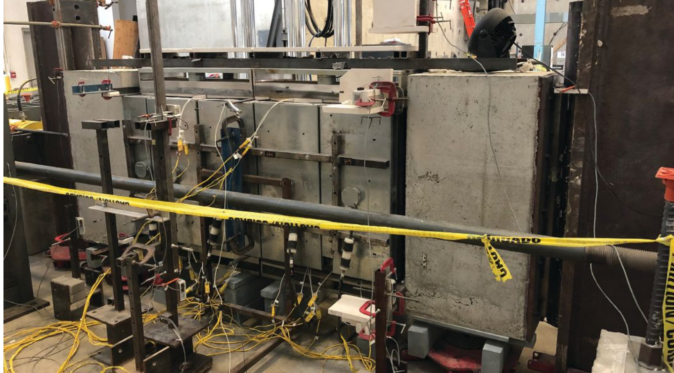
Fig. 9. A SpeedCore specimen being tested under combined elevated temperature and axial loading at Purdue University.
