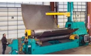
2" x 12' plate roll can roll 40' lengths
