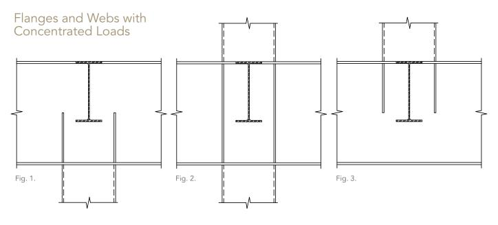
Looking at Figure 1, should web compression buckling be checked per the requirements of Section J10.5 of the AISC Specification for Structural Steel Buildings (ANSI/AISC 360)?
