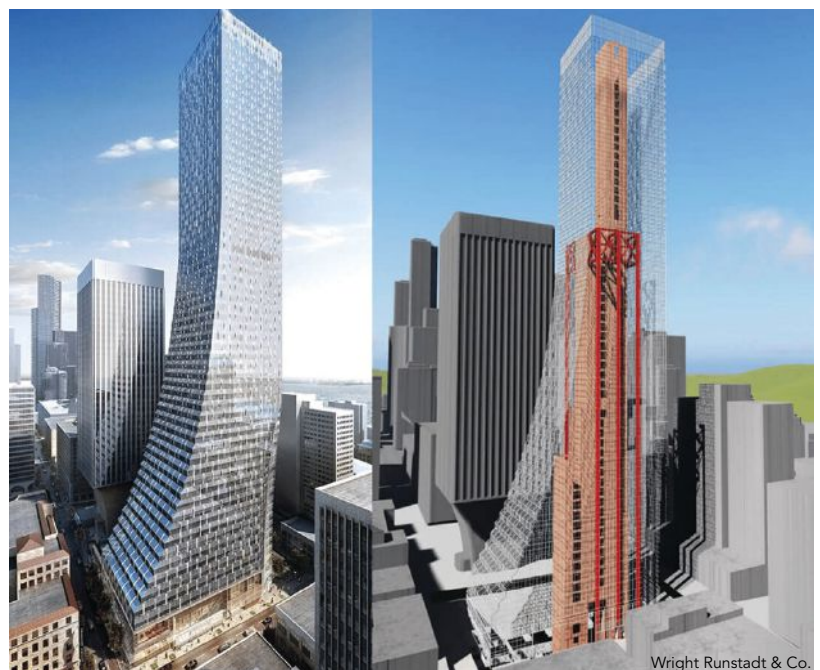
Fig. 4. A 3D rendering of Rainier Square, designed by Magnusson Klemencic Associates (MKA), in Seattle. You can read about the project, a 2022 AISC IDEAS 2 Award winner, in the May 2022 issue ( www.modernsteel.com ).
