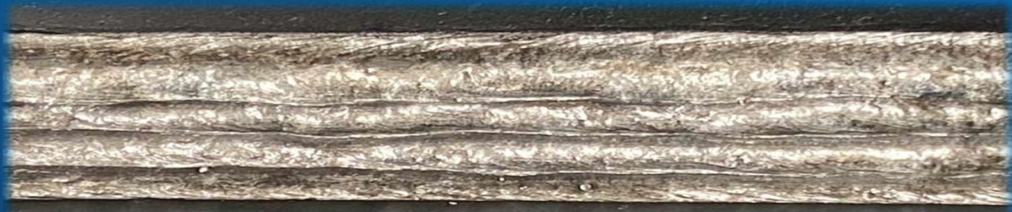
Photo: Bead appearance of DW-50AY (Multipass, Horizontal fillet welding)
