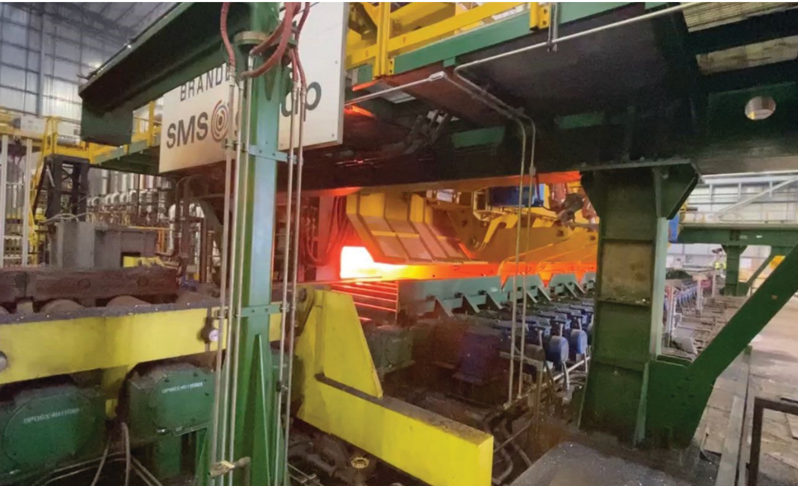
Slabs are reheated to begin the rolling process.
