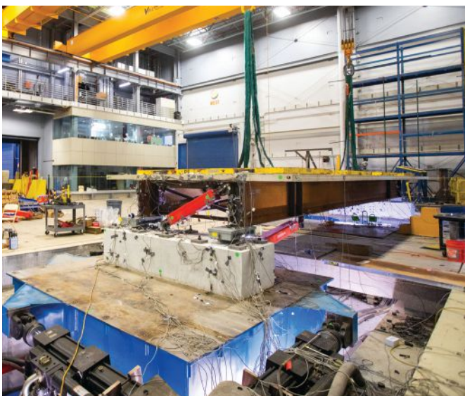
Resilient bridge concept with bi-directional diaphragms tested on two shake tables at the University at Buffalo.
