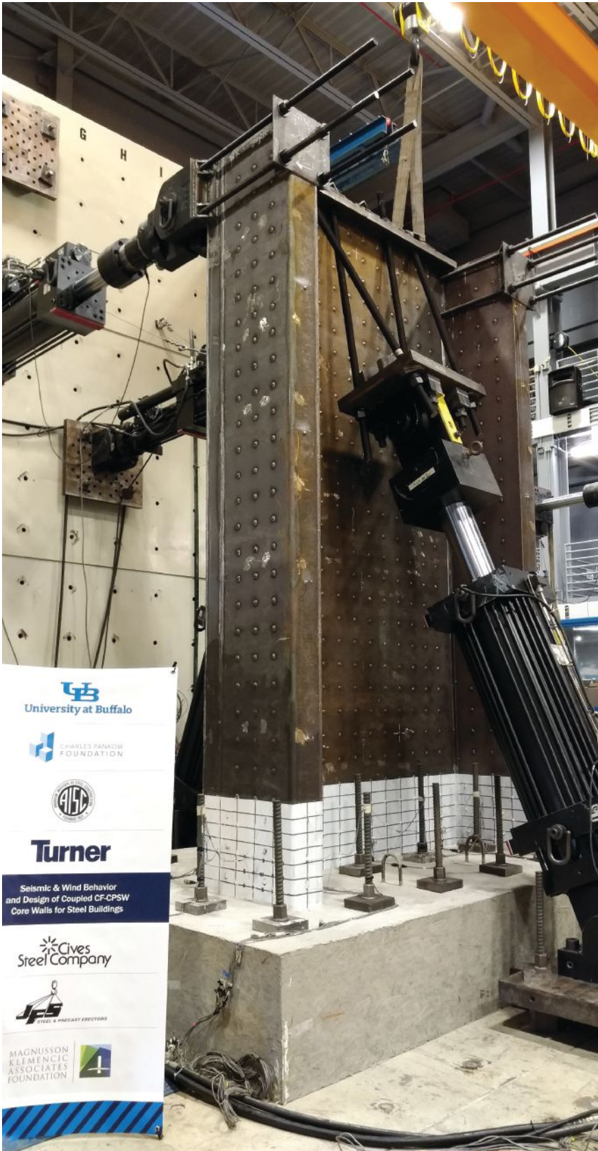
A SpeedCore specimen being tested at the University at Buffalo.
