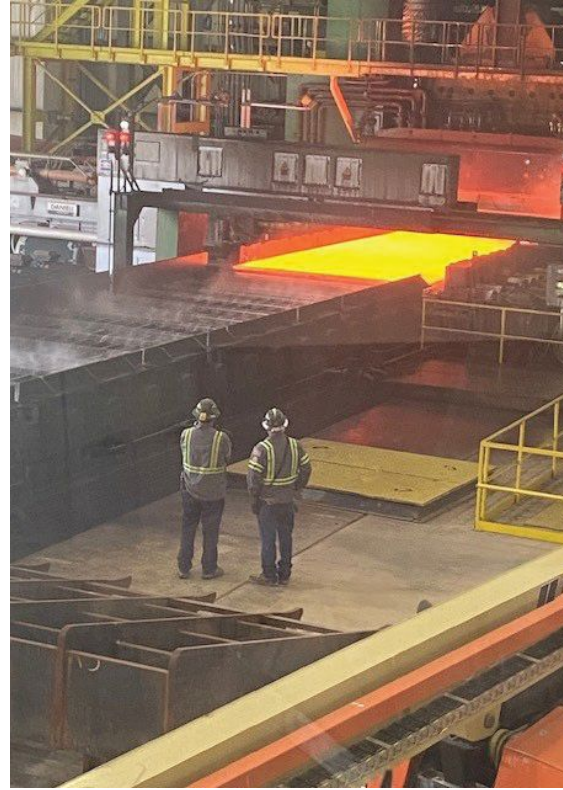
A slab enters the roughing mill.
