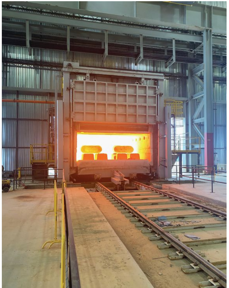
Slabs and ingots are reheated at the start of the rolling mill.
