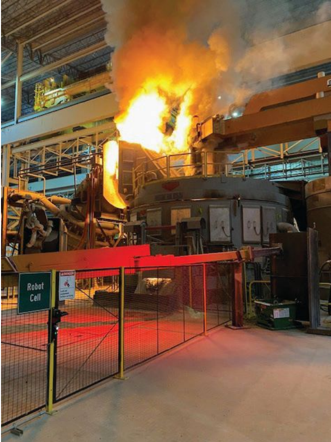
left and below: Scrap metal is melted in the electric arc furnace.
