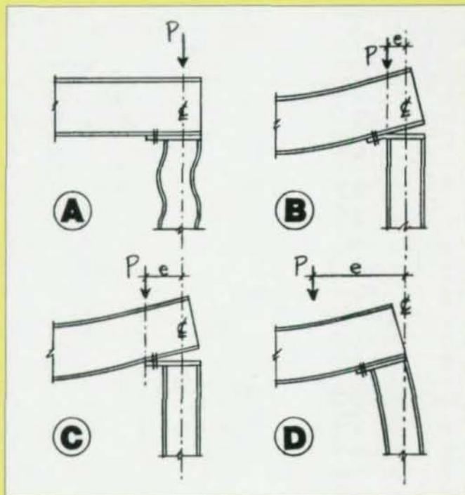
provide a system complex enough for illustrative purposes. In the hypothetical detail shown, the eccentricity is a function of the designed relative stiffness of the various components.
