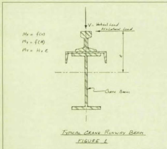
load and of the crane trolley) is applied at the top of rail. This horizontal force (see Figure 1) will result in a moment in the weak axis ( $M_y$ ) and a torsional moment ( $M_t = He$ ). In absence of the torsional moment, the beam would be checked for combined stresses as follows:
