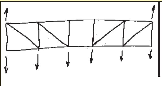
Theoretically, all joints for trusses are assumed to be pinned connections, so this truss without diagonal member in the center panel is virtually a mechanism instead of a structure. Besides, there is no force (there is no need for the diagonal member in this case) on the diagonal member only if the loading condition is perfectly symmetrical, this situation is too ideal in practice, so there is need for the diagonal member to make a stable truss design.
