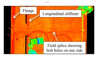
Figure 3: Laser Scan of Field Splice
