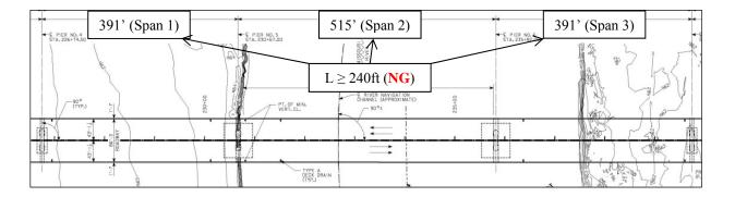
Figure 9: Plan View Showing Violations of AASHTO LRFD Approximate Equation Criteria
