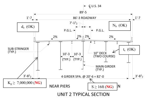
Figure 8: Typical Section Showing Violations of AASHTO LRFD Approximate Equation Criteria
